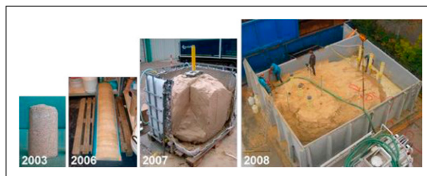
Figure 8. Scaling up from 10 cm to 100 m 3 biological sandstone. Photos: Deltares, TU Delft & Volker Wessels.
